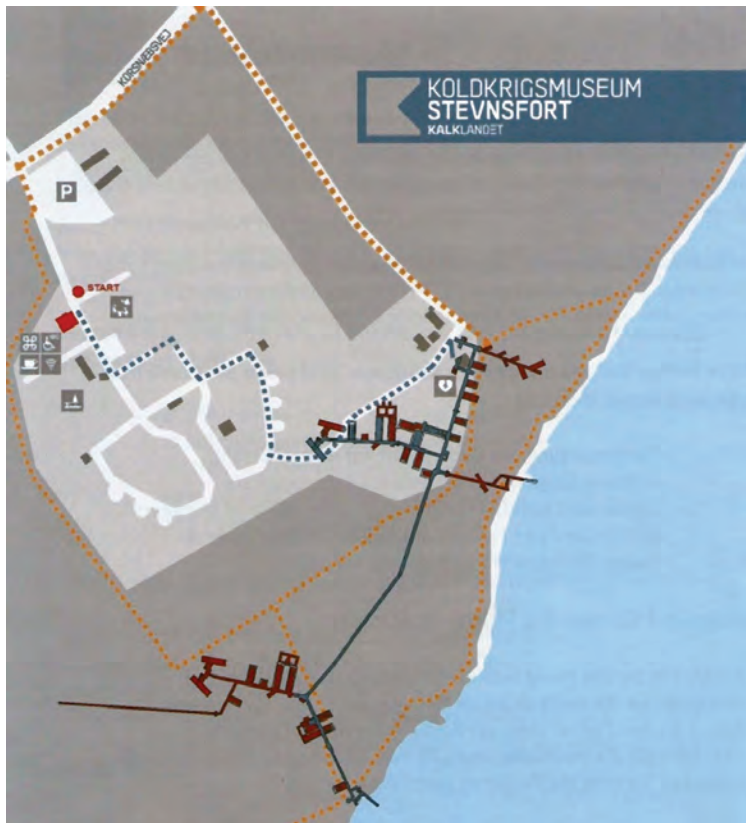
Plan of Stevns Fort. The white tracks are the surface anti-aircraft battery and the grey lines show underground passages. Underground rooms magazines, barracks etc are in brown. You can see the fort is effectively two separate batteries, with one linking corridor. The theory was that a single strike would never take out both gun positions
